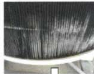
Adhesion of silica six month after the installation of the Vulcan
