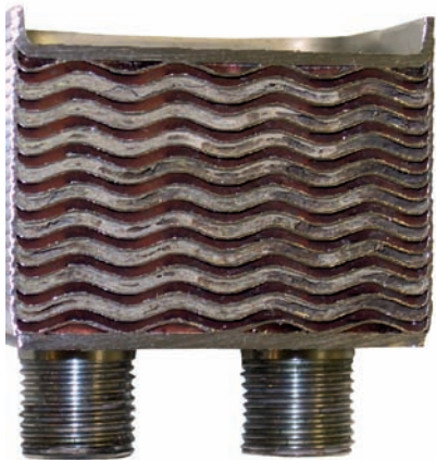
Calcified heat exchanger
