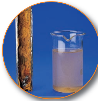
Before: Pitting, rust and brown water
