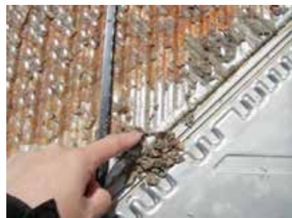
The scale on the plate heat exchanger becomes soft.
