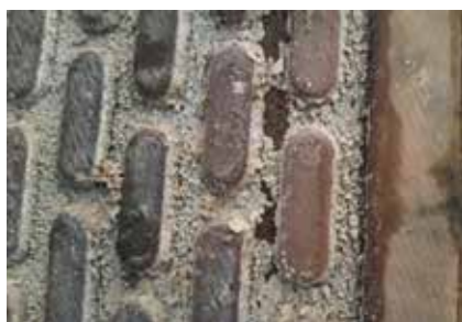
After Vulcan was installed only for 1 month, the scale is softened and falling off.
